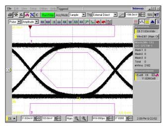
Figure 8. Eye diagram displayed on a digital sampling oscilloscope. Scattered dots above and below the main lines are evidence of baseline wander.
