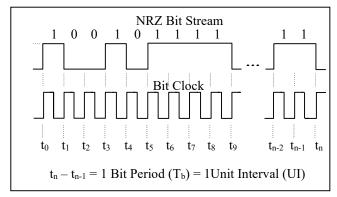
Figure 1. NRZ encoded bit stream
