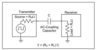
Figure 4. AC-Coupled Transmission System
